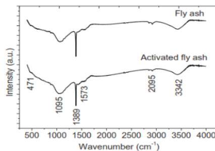
Gambar 5. Hasil Spektra FTIR adsorben fly ash
